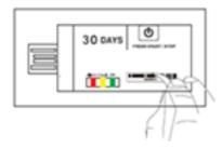
3 – **LANDING**: Press the "START / STOP" button and hold for 5 seconds, until the red LED flashes 3 times. This means that the Wise -USB Thermograph has ended the Temperature recording cycle.
